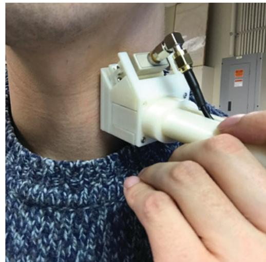
▲ Figure 1: The prototype ultrasound system and transducer assembly. The system is capable of sufficient data rate to display blood flow and arterial pulsation simultaneously. Ultrasound gel pad is utilized to achieve acoustic coupling between the transducer surface and the skin.
