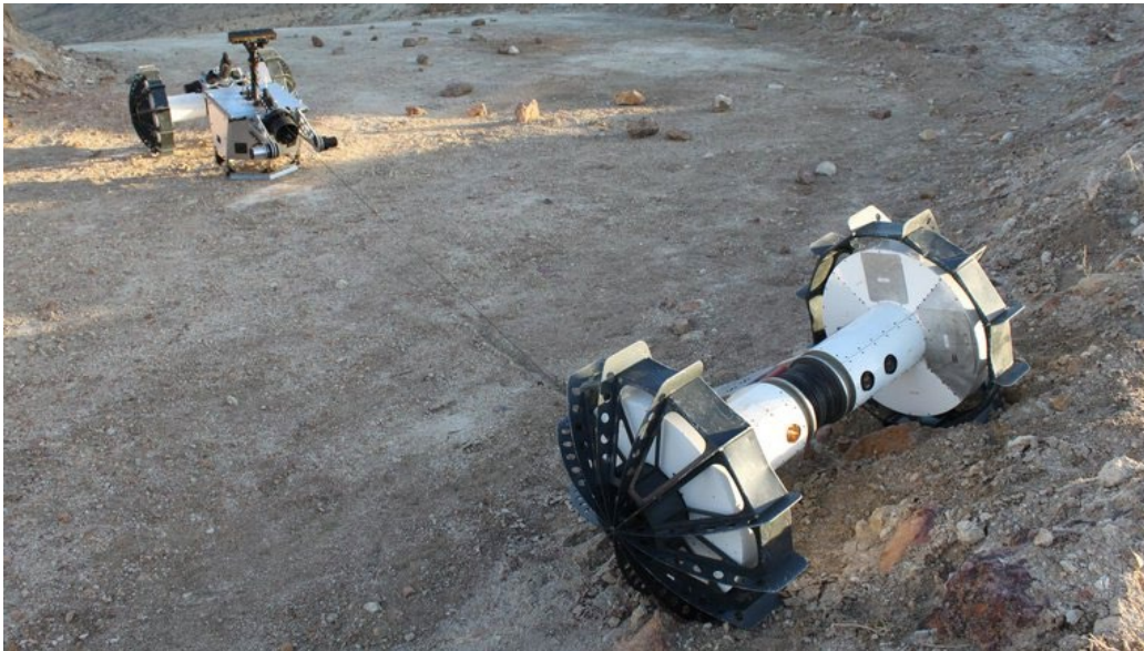
DuAxel with retractable tether [2]
