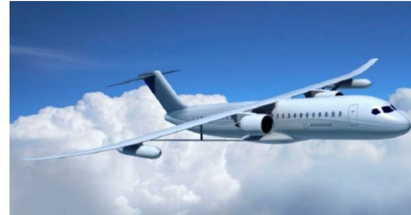
Boeing Sugar Volt, parallel hybrid 150 passenger aircraft [5].
