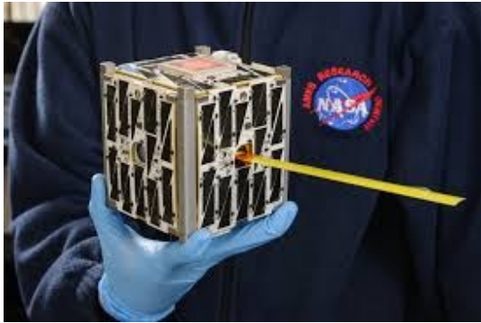
(a) CubeSat hardware ( 10\text{cm} \times 10\text{cm} \times 10\text{cm} )
