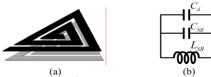
Fig.14: (a) Layout of the BCTSR (dark region denotes BCTSR etched on signal plane, and light region denotes broadsides coupled triangular SR etched on ground plane) (b) equivalent lumped circuit
