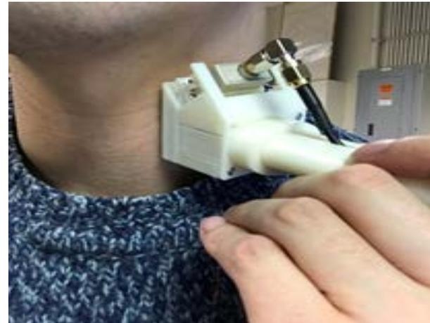
▲ Figure 2: Ultrasound transducer placed above the carotid artery.
